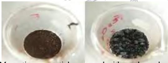
**Figure 1.** Magnetic nanoparticles covered with a polysaccharide vs magnetic nanoparticles
