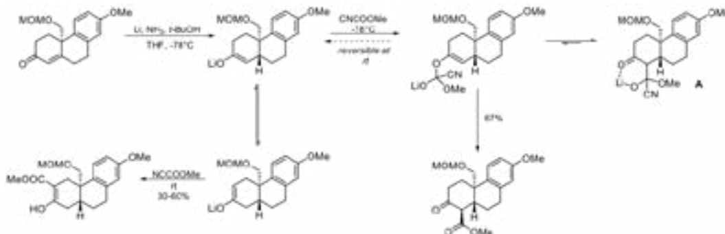
Scheme 1: C-carboxymethylation stabilization by dioxo-metalocycle (A) formation.
